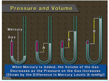
When Boyle added mercury to a closed tube containing a gas, the gas's volume decreased at a proportional rate.
