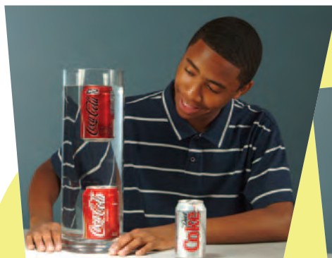
Wow—density in action! Regular Coke sinks, but the new C2 (half-the-sugar cola) floats because its overall density is less than water ( < 1.0 \text{ g/cm}^3 ).
