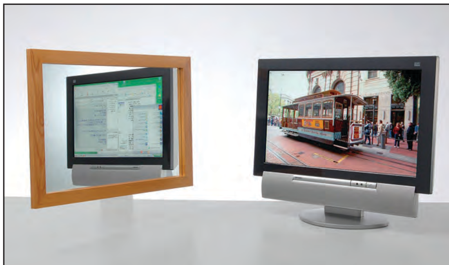
Two-way viewing angle LCD. This new LCD from Sharp Corporation sends the light from the backlight to the right and the left, making it possible to show two different images at the same time. Reflecting the LCD in a mirror shows that one user sees a TV show, while another sees an Internet homepage. One possible application is a car display that shows the driver a map, while the passenger watches a movie on DVD.
