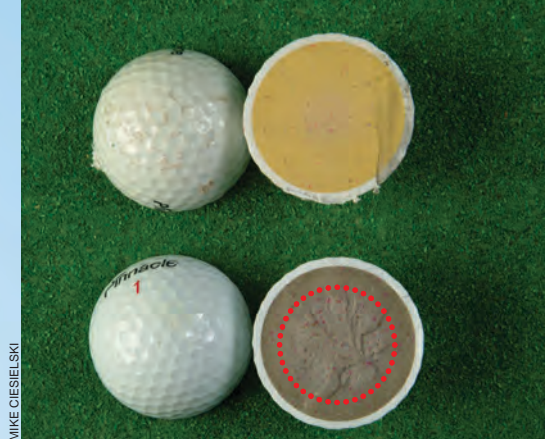
What’s in your golf ball? Both of these modern golf balls have an outer layer of Surlyn. If you look closely at the bottom ball, you will see an additional ring for the softer inner core. The manufacturer claims this design reduces spin and helps the ball fly in a straight path.
