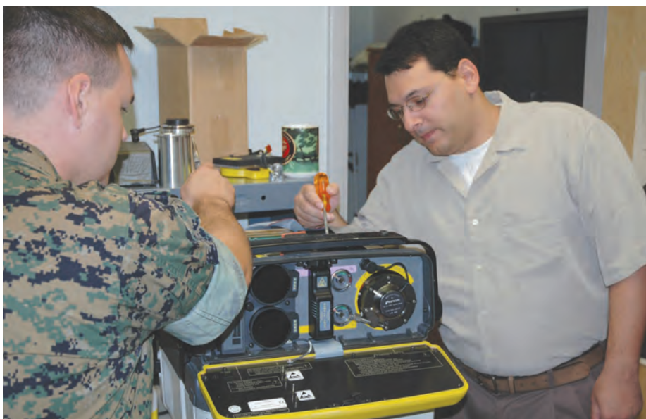
Erick Swartz and a marine are working on a portable gas chromatograph-mass spectrometer.
