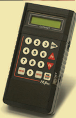
The CorTemp system can measure and record the body temperature and/or heart rate of many athletes on the field during practices or competition. Once the probe is inside the gastrointestinal tract, a crystal sensor vibrates at a frequency relative to the temperature of the body tissues surrounding it. These data are then transmitted harmlessly through the body to the monitor.
