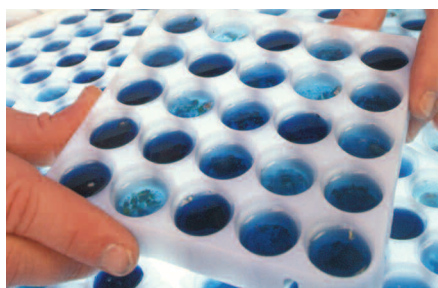
A qualitative test for GM corn. Hybrid corn samples turn test solution dark blue, while normal kernels do not.
