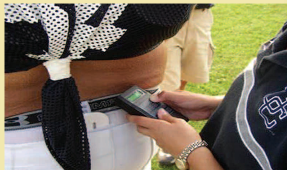
The CorTemp system can measure and record the body temperature and/or heart rate of many athletes on the field during practices or competition. Once the probe is inside the gastrointestinal tract, a crystal sensor vibrates at a frequency relative to the temperature of the body tissues surrounding it. These data are then transmitted harmlessly through the body to the monitor.
