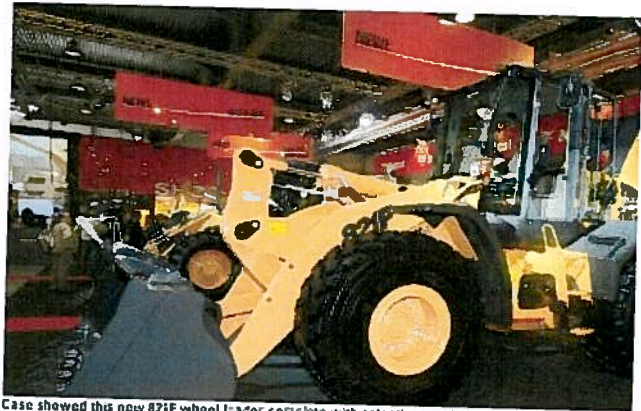
Case showed this new 821F wheel loader complete with selective catalytic reduction (SCR) technology and an AdBlue tank.
