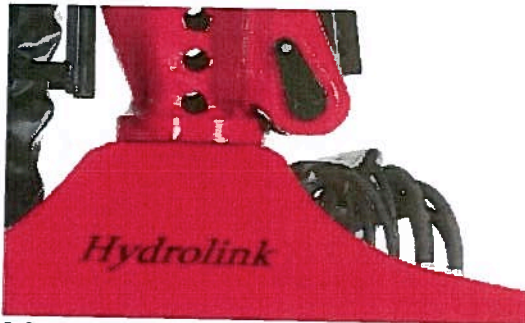
In Penz 'Hydrolink' cranes, main column bearing is packed with grease and all hydraulic service pipes are routed internally to allow for full 360-degree rotation - a major operational advantage
